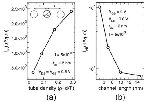
Fig. 6. (a) On-current as a function of the nanotube normalized-density per unit length  $\rho = d/T$  for a double-gate CNT-FET with  $L = 15$  nm. (b) Off-current as a function of the channel length for a double-gate CNT-FET.
