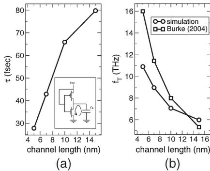
Fig. 13. (a) Inverse of the intrinsic device speed, defined as  $\tau = C_G V_{DD} / I_{on}$  as a function of the channel length for double-gate CNT-FET, where  $V_{DD} = 0.8$  V and  $C_G$  is the gate capacitance. (b) Cutoff frequency as a function of the gate length, for the double-gate CNT-FET.  $t_{ox} = 2$  nm, and  $f = 5 \times 10^{-3}$ .
