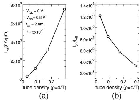
Fig. 7. (a) Off-current as a function of the nanotube normalized-density per unit length  $\rho = d/T$  for a double-gate CNT-FET with  $L = 15$  nm. (b)  $I_{on}/I_{off}$  ratio as a function of the nanotube normalized-density per unit length  $\rho = d/T$  for a double-gate CNT-FET with  $L = 15$  nm.
