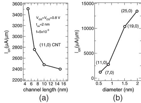
Fig. 5. (a) On-current per unit width as a function of the channel length for a double-gate CNT-FET (2-nm lateral dielectric between adjacent nanotubes). (b)  $I_{on}$  current per nanotube as a function of the nanotube diameter, for an  $L = 7$  nm double-gate CNT-FET.  $t_{ox} = 2$  nm, and  $f = 5 \times 10^{-3}$ .
