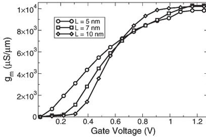
Fig. 11. Transconductance as a function of the gate voltage for double-gate CNT-FETs with different channel lengths:  $L = 5, 7,$  and  $10$  nm;  $t_{ox} = 2$  nm;  $V_{DS} = 0.8$  V; and  $f = 5 \times 10^{-3}$ .
