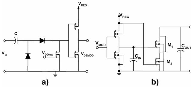
Figure 4. a) Demodulator; b) Modulator.
