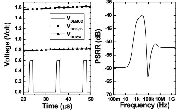
Figure 3. Left: Output signal of the demodulator and the voltage multiplier with a PWM signal at the antenna. Right: PSRR of the voltage regulator.
