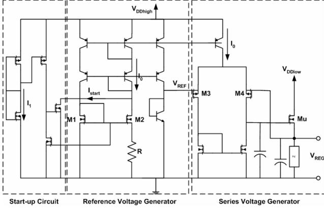
Figure 2. Circuit of the Voltage Regulator
