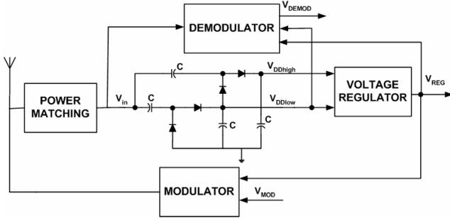
Figure 1. Architecture of the RF Section.
