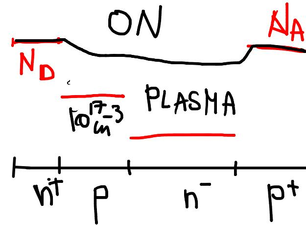
$$V_{ON} = V_J + R_d I + V_{CESAT} \approx 2V$$
