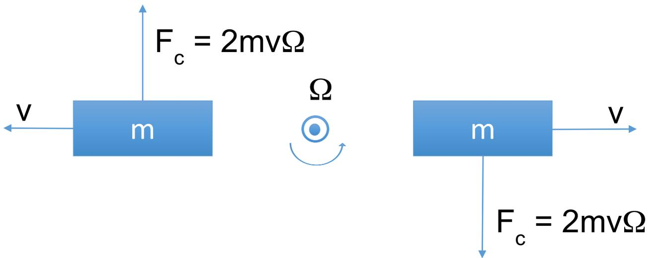
Let us assume that the structure rotates with angular velocity  $\Omega$  in the plane, as indicated in the figure.
