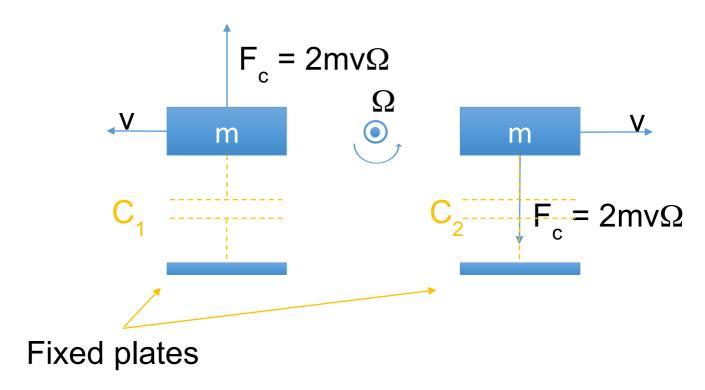
This differential structure is required in order to eliminate the effect of a linear acceleration (because a linear acceleration would have the same effect on both capacitances and therefore  $\Delta C$  would be zero.
