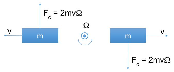
Let us assume that the structure rotates with angular velocity W in the plane, as indicated in the figure.
