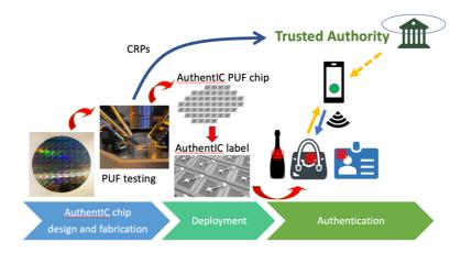
As part of the European **AUTHENTIC** research project, we are working on the design of mixed-signal integrated circuits for secure cryptographic key distribution based on logic-inmemory circuits. In this thesis, we focus on the design of a high entropy physical unclonable function (PUF).
