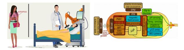
As part of the European **AUTOCAPSULE** research project, we are working on the development of a wireless robotic capsule for colonoscopy. In particular we are developing the full electronic subsystems for wireless power transfer, wireless communication, sensor data conditioning. This thesis deals with the wireless power transfer subsystem.
