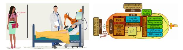
As part of the European **AUTOCAPSULE** research project, we are working on the development of a wireless robotic capsule for colonoscopy. In particular we are developing the full electronic subsystems for wireless power transfer, wireless communication, sensor data conditioning. This thesis deals with the wireless communication subsystem.
