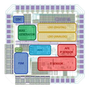
As part of the European **CHARM** research project, we are working on sensors in extremely challenging industrial environments. In particular we want to develop high temperature and pressure sensors industrial applications, pushing standard CMOS technology up to 300 C (above the normal operating range) with the use of temperature-compensation techniques.
