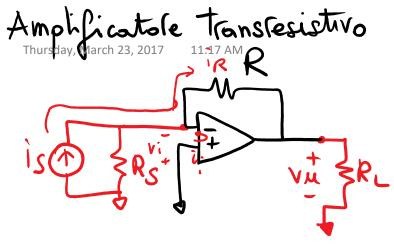
$$i_{R} = i_{S} - \frac{v_{i}}{R_{S}} + i_{i} = i_{S}$$
