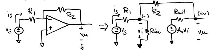
$$-\frac{V_{1}}{R_{1}} \left( \frac{\Lambda}{R_{1}} + \frac{\Lambda}{R_{im}} + \frac{\Lambda}{R_{2}} \right) - V_{S} \frac{\Lambda}{R_{\Lambda}} - V_{M} \frac{\Lambda}{R_{2}} = 0$$
