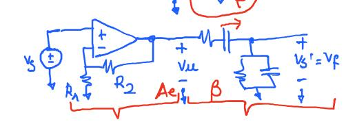
$$Ae = \frac{Vu}{VS} = \left(1 + \frac{R_2}{R_1}\right)$$
